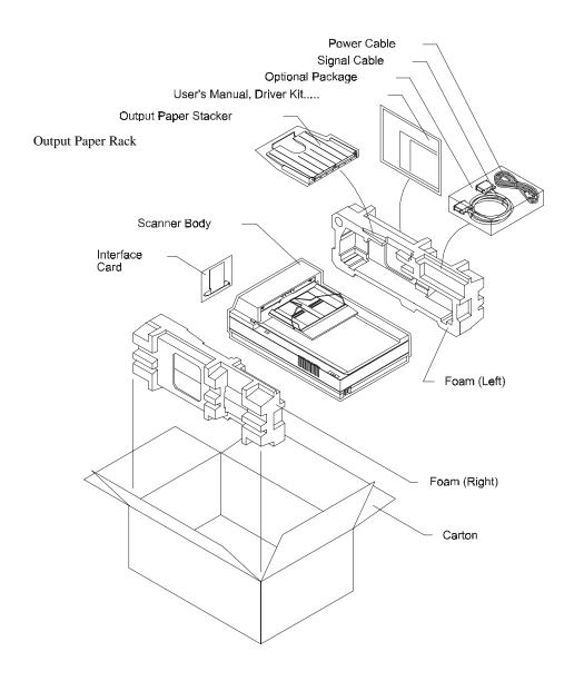
Figure 1-1 Scanner packing
